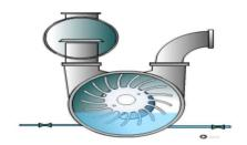
A vacuum pump is a device that draws gas molecules from a sealed volume in order to leave behind a partial vacuum. The job of a vacuum pump is to generate a relative vacuum within a capacity. The first vacuum pump was invented in 1650 by Otto von Guericke, and was preceded by the suction pump, which dates to antiquity
