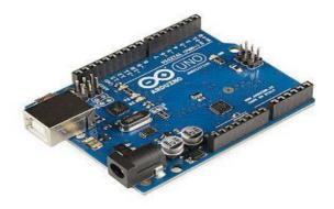
Arduino is a single-board microcontroller to make using electronics in multidisciplinary projects more accessible. The hardware consists of an open-source hardware board designed around an 8-bit AtmelAVR microcontroller, or a 32- bit Atmel ARM. The software consists of a standard programming language compiler and a boot loader that executes on the microcontroller.
