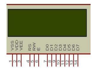
Crystalonics dot –matrix (alphanumeric) liquid crystaldisplays are available in TN, STN types, with or without backlight. The use of C-MOS LCD controller and driver ICs result in low power consumption. These modules can be interfaced with a 4-bit or 8-bit micro processor /Micro controller.
