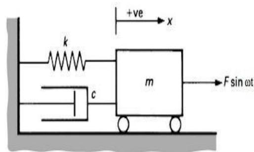
Fig 1: Damped Harmonic Oscillator
