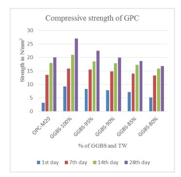
It has been observed that there is an increase in compression strength while increase in percentage of GGBS and reducing the % of tannery waste and has been illustrated with the above bar chart with samples having different proportions with different ages of 1<sup>st</sup>, 7<sup>th</sup>, 14<sup>th</sup>, 28<sup>th</sup> day of curing respectively in room temperature.
