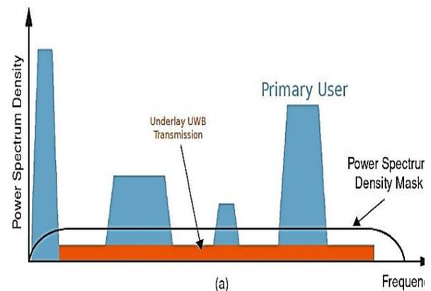
Figure 1: Details of Cognitive Radio Underlay model
