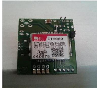
GSM (Global System for Mobile communication) is a digital mobile telephony system that is widely used in Europe and other parts of the world. GSM uses a variation of time division multiple access (TDMA) and is the most widely used of the three digital wireless telephony technologies (TDMA, GSM, and CDMA). GSM digitizes and compresses data, then sends it down a channel with two other streams of user data, each in its own time slot. It operates at either the 900 MHz or 1800 MHz frequency band.
