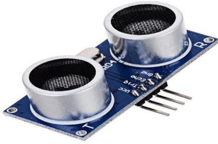
Ultrasonic sensors are used for distance measuring applications. These gadgets regularly transmit a short burst of ultrasonic sound to a target, which reflects the sound back to the sensor. The system then measures the time for the echo to return to the sensor and computes the distance to the target using the speed of sound within the medium.
