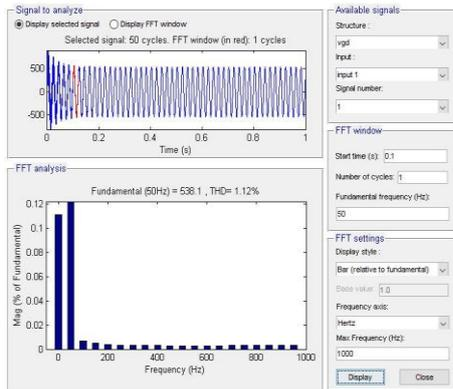
Figure 16: %THD in Voltage waveform without DVR
