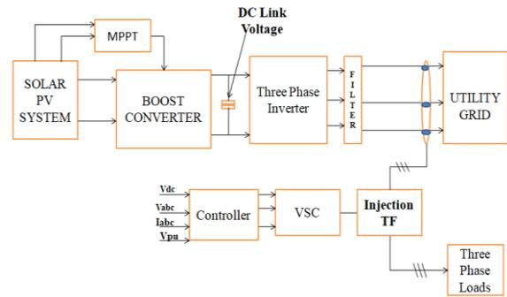
Figure 1: Block Diagram of Grid tied Solar PV with DVR
