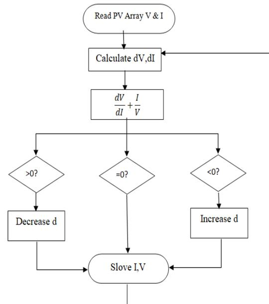
Figure 4: Flow Chart of Incremental Algorithm Conductance
