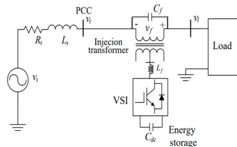
Figure 2: DVR schematic diagram
